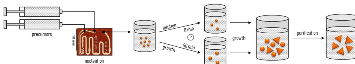
Figure 1. The representation of gold nanotriangle synthesis implementing a microfluidic setup
